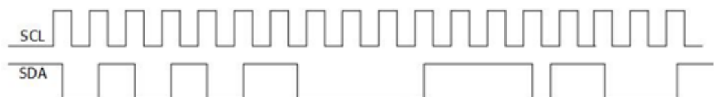
Figure 14.4 Schematic diagram of I2C serial bus
