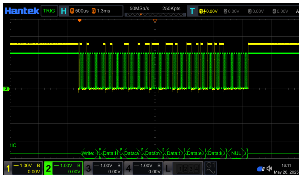
Figure 14.5 I2C decoding example
