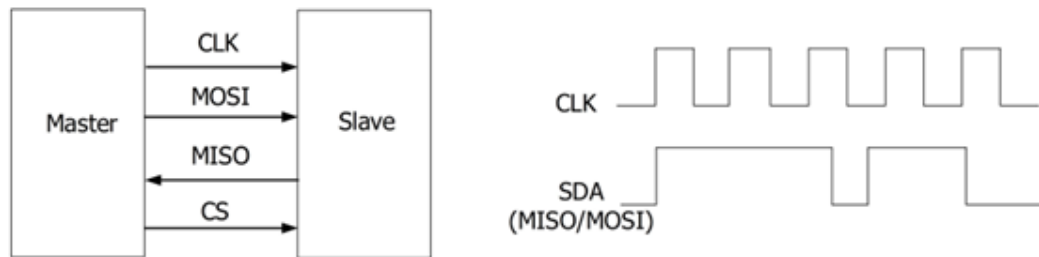
Figure 14.6 SPI Bus Schematic
